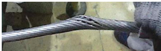
Strand distortion due to “concentrated” overtwisting (270° rotation squeezing of 1 m specimen)
